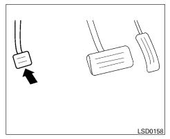
To engage: Firmly depress the parking brake.
